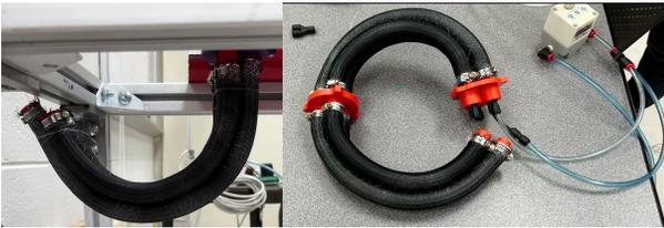
Fig. 3. Maximum bending for single-section (left) and multi-section (right).
