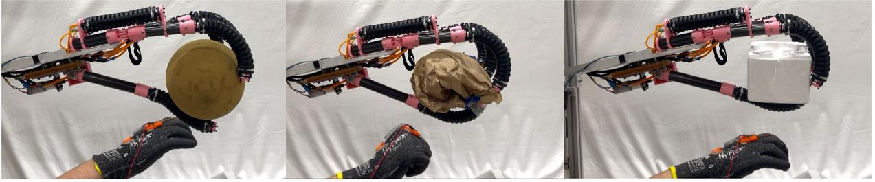
Fig. 8. The CLAW grasping the balloon, packing sheet, and a piece of foam following the operator’s hand motion.
