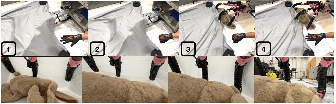
Fig. 10. Screenshots of the CLAW performing the rescue task 1, where it crawls underneath the bedsheet via the mobile platform (1), located and grasped the plush animal (2 and 3), and moved it to safety (4). The second row shows the first-person perspective view of the CLAW.
